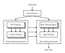
Figure: BeatRoot System Schematic (Dixon 2006a)
