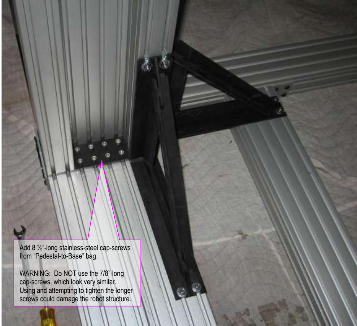
Figure 12 – Pedestal Anchoring
