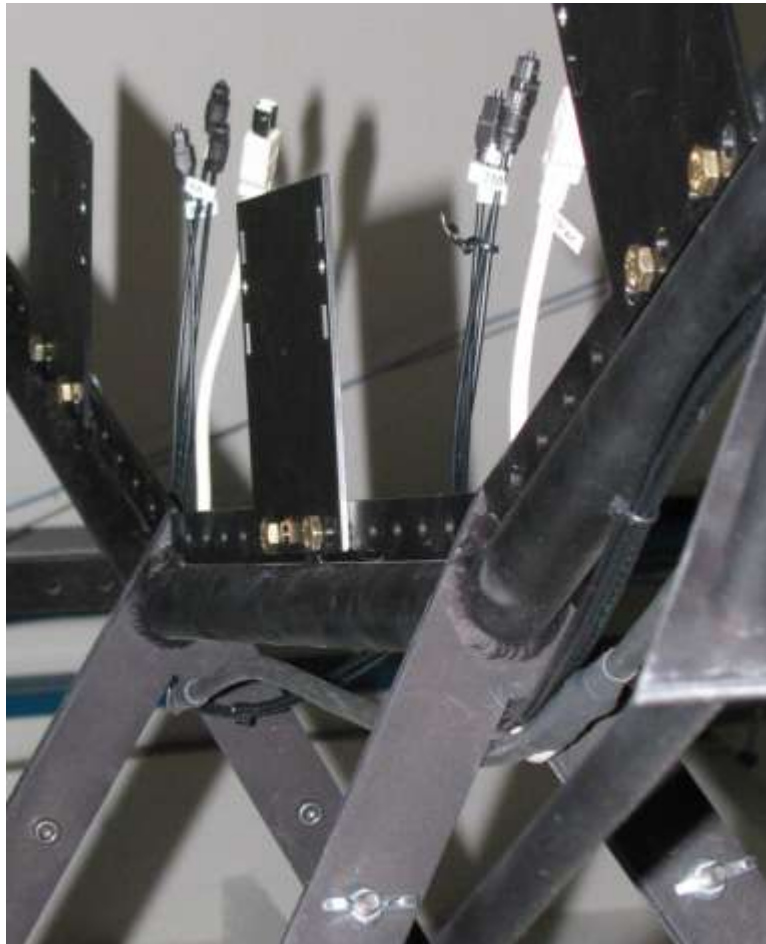
Figure 24 – Gusset Mounting on Arc Segment dorsal tube.
