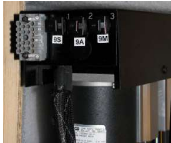
Figure 19 – Horizontal axis gear box connections. Shown with Toslink covers in place.
