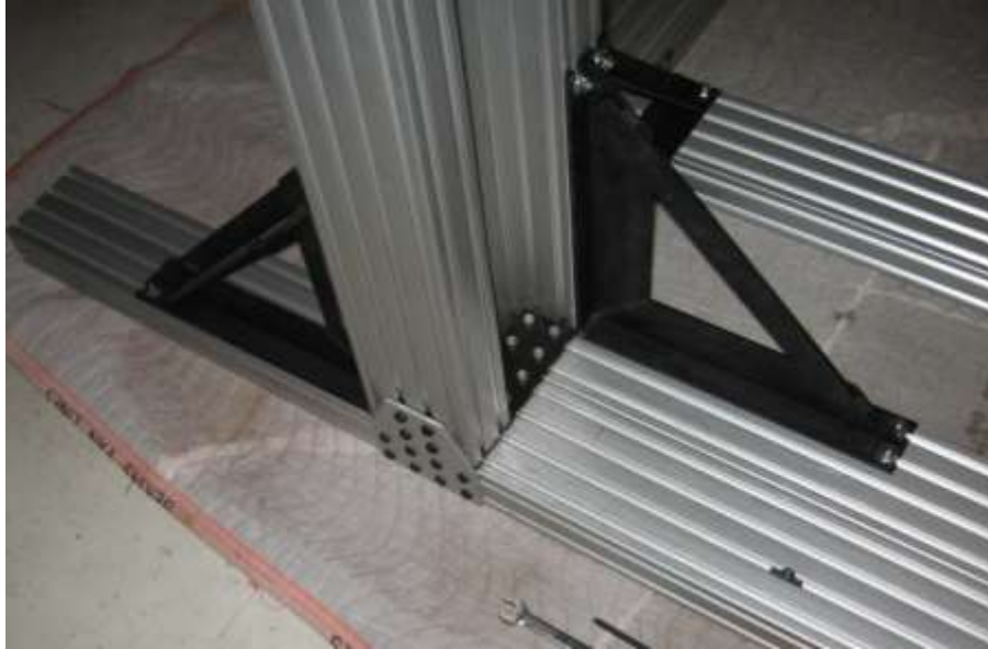
Figure 8 - Assembled Pedestal with angle brackets
