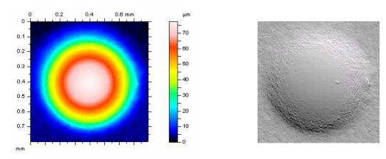
"Distance" image (false color) and "Intensity" image (rendered image) of a microlens
