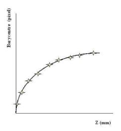
The relation between the position of the spectral peak ("barycenter" in pixels) and the axial position of the object ("distance" in µm) is called "calibration lookup table" (LUT).
