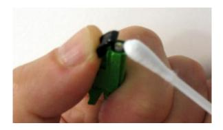
Raise the black protecting cap over the fiber optics plug, and clean the fiber optics tip carefully. Use absorbent cotton, or a paper towel, soaked with alcohol (e.g. Ethanol or Methanol). Perform circular movement so as to push the dust grains away from the fiber tip.
