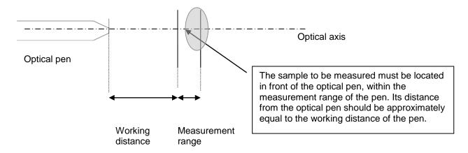
As soon as the sample is located inside the measuring range of the optical pen, the "Measurement" LED indicator on the sensor front panel lights on. Once the sample is inside the measuring range, use the "Measurement" LED indicator color to adjust its position at the center of the measuring range:
