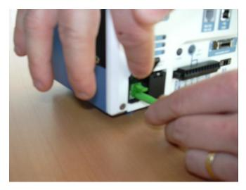
To remove the fiber optics from its socket, first press on the locking lever, then pull the lead out of the socket.
