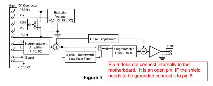
Figure 4 is the Model 136 block diagram.
