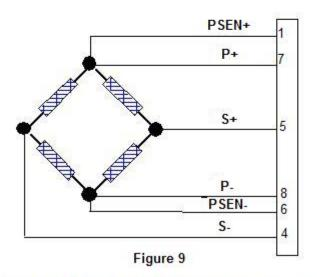
Typical Bridge Connection with remote excitation sensing
