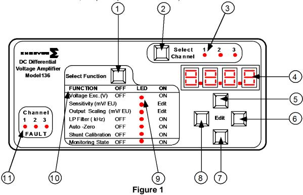
Figure 1 Items 5, 6, 7, and 8 correspond, respectively to the "Up", "Right", "Down" and "Left" Edit push buttons. These push buttons are used to change the entries on the digital panel meter and are used in conjunction with the appropriate "Select Function" parameter to be programmed. (See Section 2.4, Operation and sub-sections contained, for specific push button abilities.)
