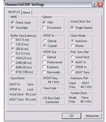
SyncCheck indicates whether there is a valid signal (Lock, No Lock) for each input (Word Clock, ADAT, SPDIF), or if there is a valid and synchronous signal (Sync). The AutoSync Ref(erence) display shows the input and frequency of the current sync source.
