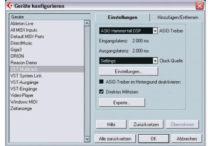
notes placed close before or behind the correct position), the settings in Cubase/Nuendo have to be changed. At the time of print, the best settings are the use of emulated MIDI driver/ports, and the activation of the option 'Use System Timestamp'.
