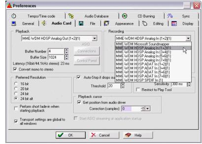
The HDSP system's ADAT optical interface allows sample rates of up to 96 kHz using a standard ADAT recorder. Single-channel data at this frequency requires two ADAT channels, achieved using the *Sample Multiplexing* technique. This reduces the number of available ADAT channels from 8 to 4. Under Windows MME, channels are routed to ADAT devices in double-speed mode as follows:
