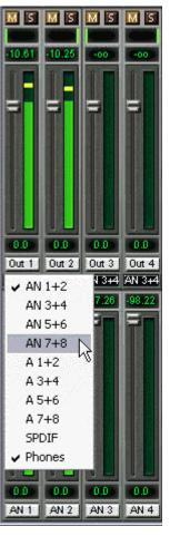
You will certainly have noticed that the signal at the outputs 7/8 did not change while you were routing channel 4 to other outputs and setting different gain values for those. With all analog and most digital mixing desks, the fader setting would affect the level for every routed bus - not so for TotalMix. TotalMix allows for setting all fader values individually. Therefore the faders and the panpots jump to the appropriate setting as soon as another routing is chosen.
