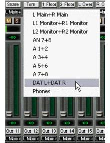
The hardware outputs (third row) can be edited in the same way. In this case, the names in the routing drop down menus will change automatically. Additionally the names in the drop down menus of the Monitor section will change as well.
