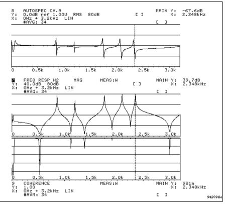
Fig. 1 (top) Input force spectrum for pseudo-random excitation. (Bottom) Frequency Response Function and Coherence using pseudo-random excitation. (Measurement performed using the Type 5961 with the Multichannel Analysis System Type 3550)
