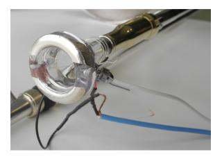
FIG. 1. (Color online) Kelly plastic mouthpiece 6 1/2 AL with two silverplated electrodes mounted on the rim. The downstream microphone is mounted to record the acoustic pressure in the mouthpiece cup.
