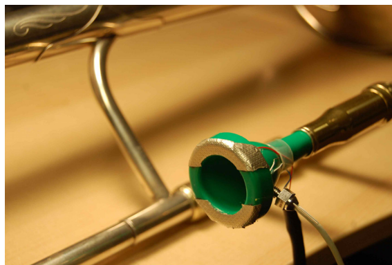
Figure 1: Lip conductance sensor and pressure transducer embedded in a plastic trombone mouthpiece and mounted on a King 2102 Silver Sonic tenor trombone.
