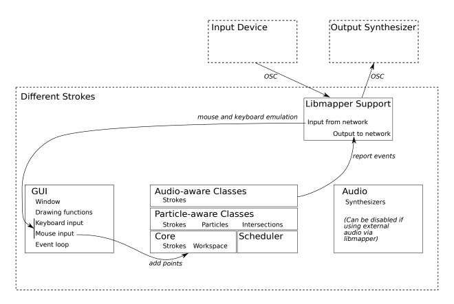
Figure 6.2 A system diagram for *libmapper* integration into *Different Strokes*.
