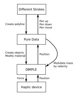
Figure 5.4 Information flow between the DS and DIMPLE applications.
