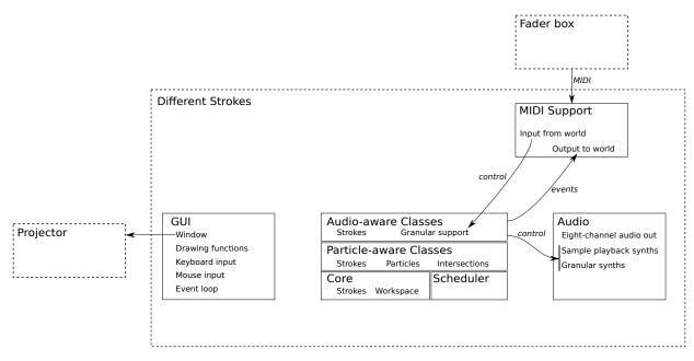
**Figure 4.11** System diagram illustrating the new features added to *Different Strokes* for the *d\_verse* project.
