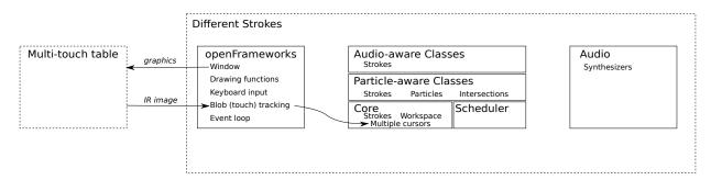
**Figure 4.13** System diagram illustrating the new features added to *Different Strokes* to support multi-touch interaction.
