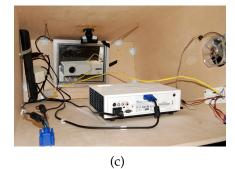
**Figure 4.14** Images of the *TactoSonix* multi-touch table. (a) The whole unit. (b) The table without the plexiglass top, showing the projector. (c) An interior view, showing the IR camera, projector and mirror. (Photos courtesy Bruno Angeles.)
