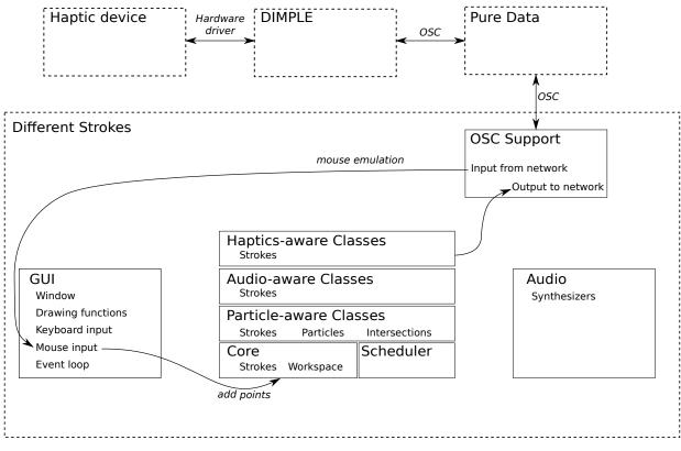
**Figure 5.2** A system diagram for DIMPLE integration into *Different Strokes* to support haptic input devices.
