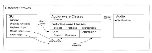
**Figure 4.5** The main components of the DS code are the graphics subsystem (GUI), the simulation subsystem, and the audio subsystem. Arrows indicate the interactions between the components. The simulation is made up of layers of classes that each add extra functionality to the one below.
