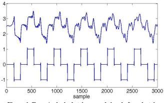
Figure 1. Top : A plucked string sound signal of an electric guitar y(n); Bottom : DW simulation of the plucked string sound,  $v_{Lp}$ .
