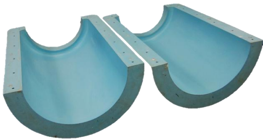
Fig. 2. The two-part GFRP mold
