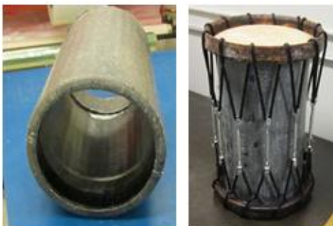
Fig.6. Finished sandwich drum shell and final assembly
