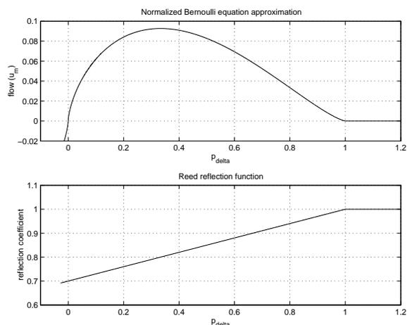
Figure 2: Bernoulli static flow expression (top); Simplified reed reflection function (bottom).
