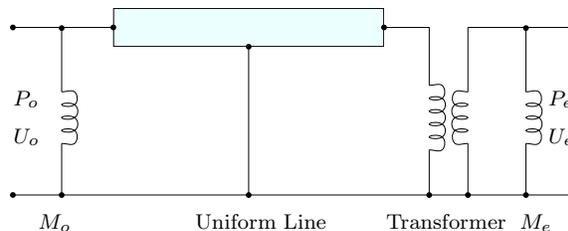
Figure 4: Equivalent circuit of a conical waveguide.
