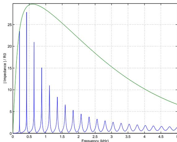
Figure 7: An example conic frustum input impedance.
