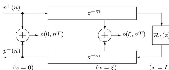
Figure 1: Digital waveguide implementation of plane-wave propagation in a cylindrical pipe, neglecting viscothermal losses.
