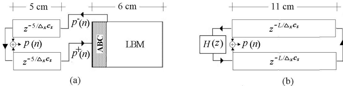
Figure 3: Different representations of a closed-closed pipe model.
