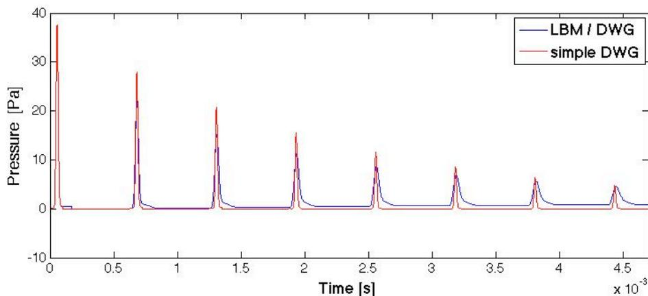
Figure 4: Impulse responses of two closed-closed pipe models.
