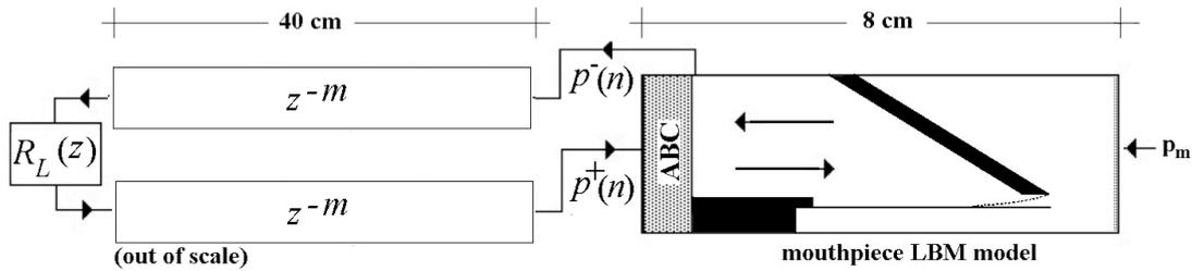
Figure 2: Scheme of the junction between a LBM grid and the DWG.
