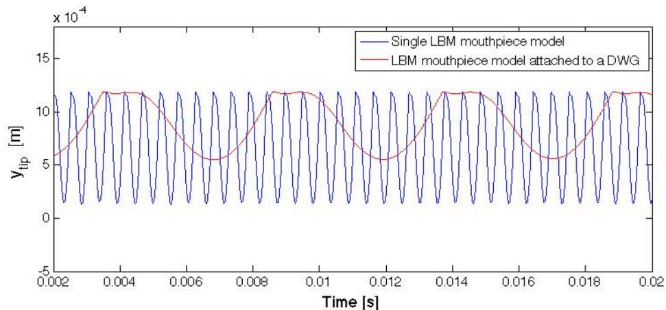
Figure 5: Time histories of the coupled and decoupled LBM mouthpiece-reed model.
