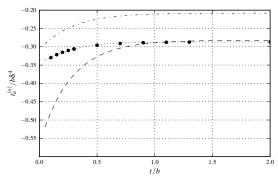
Figure 8: Series length correction  $t_a^{(o)}/b\delta^4$  as a function of t/b for  $\delta = 1.0$ . FEM results (filled circles). Data fit formula Eq. 37 (dotted). Theory: Eq. 16 (dashed), Eq. 14 (dash-dot).
