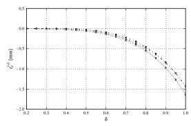
Figure 13: Series length correction  $t_a$  in mm for a tonehole on a conical bore with taper angle of 3 degrees: limit for long (squares) and short (circles) toneholes – upstream part (filled), downstream part (unfilled).
