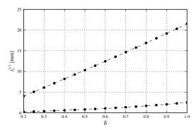
Figure 9: Shunt length correction  $t_s^{(c)}$  as a function of  $\delta$  with t/b = 0.1 (bottom) and t/b = 2.0 (top). FEM results (filled circles). Theoretical value  $(t + t_m)$  where  $t_m$  is calculated using Eq. 7 (dashed).
