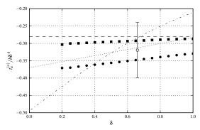
Figure 7: Series length correction  $t_a^{(o)}/b\delta^4$  as a function of  $\delta$ . FEM results: limit for large t/b (filled squares), limit for small t/b (filled circles). Theoretical formulas: Eq. 14 (dash-dot), Eq. 15 (dashed) and Eq. 16 (dotted).
