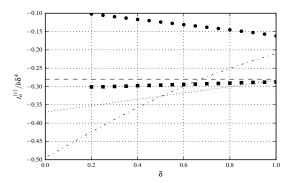
Figure 11: Series length correction  $t_a^{(c)}/b\delta^4$  as a function of  $\delta$ . FEM results: limit for large t/b (filled squares), limit for small t/b (filled circles). Theoretical formulas: Eq. 14 (dash-dot), Eq. 15 (dashed) and Eq. 16 (dotted).
