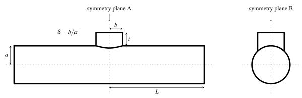
Figure 1: Diagram representing a tonehole on a cylindrical tube.
