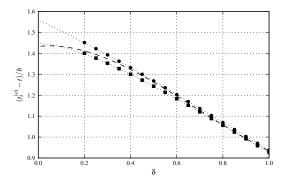
Figure 4: Difference between the shunt length correction  $t_s^{(o)}$  and the tonehole height t divided by the tonehole radius b as a function of  $\delta$ : FEM results for tall (squares) and short (circle) toneholes. Data fit formula (dotted). Current theory with Eq. 6 (dashed).
