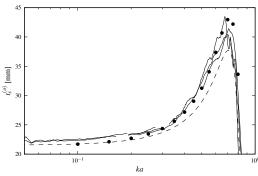
Figure 2: Shunt length correction  $t_s^{(o)}$  as a function of ka for the two toneholes studied by Dalmont et al.:  $\delta = 0.7$  and t/b = 1.3 (top graph),  $\delta = 1.0$ , t/b = 1.01 (bottom graph). FEM results (filled circles), experimental data from Dalmont et al. (solid lines) and theoretical results with Eq. 6 (dashed).
