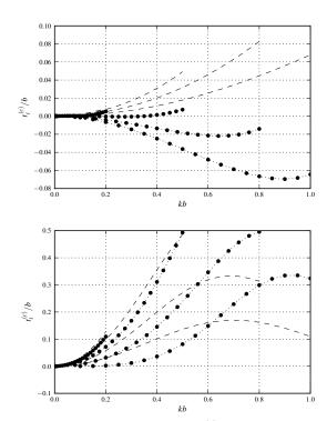
Figure 10: Inner length correction  $t_i^{(c)}/b$  for closed toneholes as a function of kb for  $\delta = 0.2, 0.5, 0.8, 1.0$  obtained from FEM simulations (filled circles) compared to theory (dashed). Top: t/b = 0.5, bottom: t/b = 2.0. The dotted line is a visual aid.
