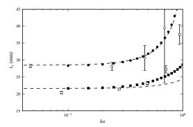
Figure 3: Shunt length correction  $t_s^{(o)}$  as a function of ka for the two toneholes studies by Keefe:  $\delta = 0.66$  and t/b = 0.48 (bottom curves),  $\delta = 0.32$  and t/b = 3.15 (top curves). FEM results: for  $\delta = 0.66$  (filled circles) and for  $\delta = 0.32$  (filled squares). Experimental data from Keefe (markers with error bar) and theoretical results with Eq. 6 (dashed).
