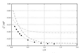
Figure 12: Series length correction  $t_a^{(c)}/b\delta^4$  as a function of t/b for  $\delta = 1.0$ . FEM results (filled circles). Data fit formula Eq. 37 (dotted). Theory: Eq. 16 (dash-dot), Eq. 14 (dashed).
