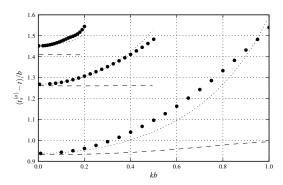
Figure 6: Difference between the shunt length correction  $t_s^{(o)}$  and the tonehole height t divided by the tonehole radius b as a function of kb for three values of  $\delta$  (0.2, 0.5 and 1.0, from top curve to bottom curve) and a value of t/b = 0.1 obtained from FEM simulations (filled circles). Current theory with Eq. 6 (dashed), new results with Eq. 35 (dotted).
