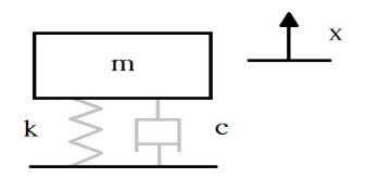
Fig. 2.3 A single harmonic oscillator
