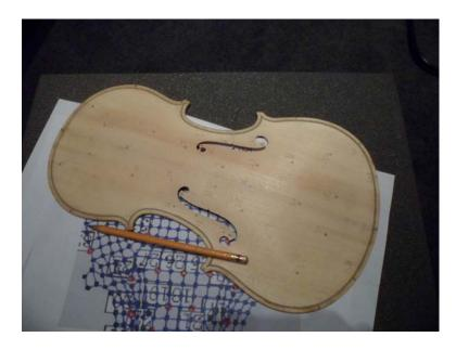
Fig. 3.12 Marked points on the spruce plate
