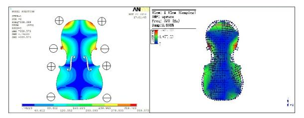
Fig. 4.9 Comparison of Mode 6 of the spruce plate by the FEM and the Modal Analysis
