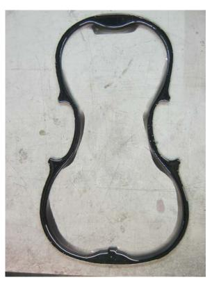
Fig. 4.16 Stage 2 of making the urethane ring
