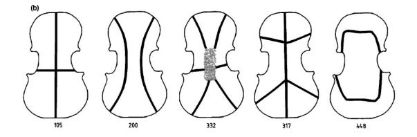
Fig. 5.2 The first six modes of the spruce plate by the FEM (Molin) [5]
