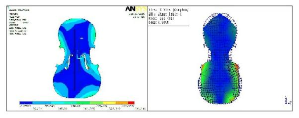
Fig. 4.21 Comparison of Mode 4 of the composite plate #1 by the FEM and the Modal Analysis
