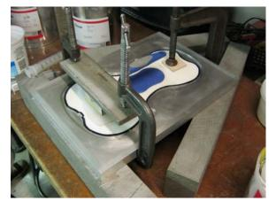
Fig. 4.15 Stage 1 of making the urethane ring
