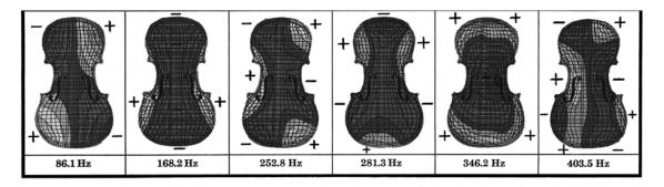
Fig. 5.1 The first six modes of the spruce plate by the FEM (Bretos) [4]
