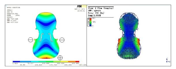
Fig. 4.5 Comparison of Mode 2 of the spruce plate by the FEM and the Modal Analysis
