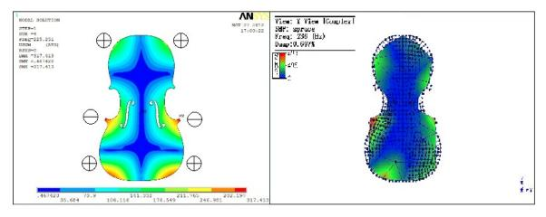
Fig. 4.7 Comparison of Mode 4 of the spruce plate by the FEM and the Modal Analysis
