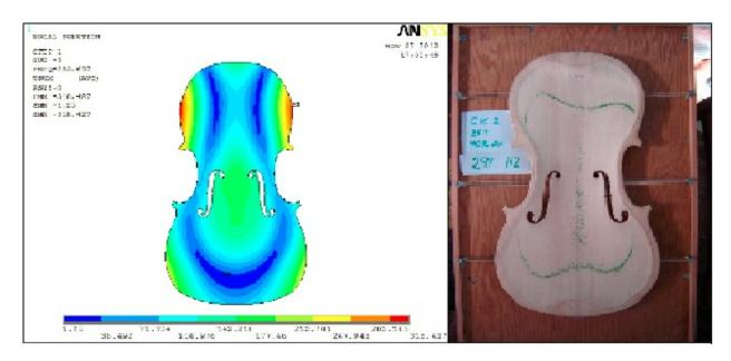
Fig. 4.3 Mode 5 of the spruce plate by the FEM and the Chladni Method
