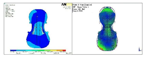
**Fig. 4.22** Comparison of Mode 5 of the composite plate #1 by the FEM and the Modal Analysis
