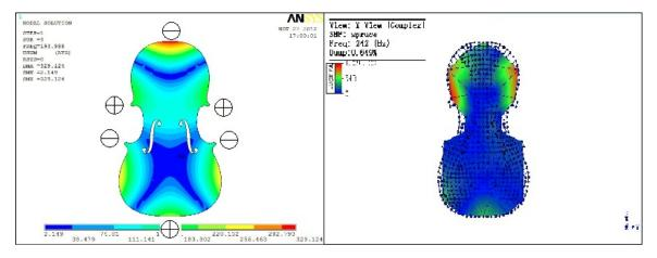
**Fig. 4.6** Comparison of Mode 3 of the spruce plate by the FEM and the Modal Analysis
