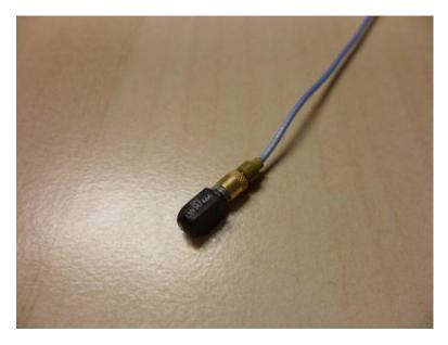
Fig. 3.10 Accelerometer Model 352C23/NC
