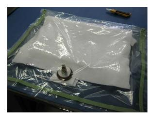
Fig. 4.11 Stage 1 of making a composite plate (layers cut and put in mould)
