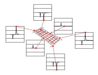
Fig. 3.16 Plate mode shape for mode 2 [3]
