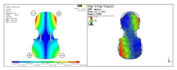
Fig. 4.4 Comparison of Mode 1 of the spruce plate by the FEM and the Modal Analysis
