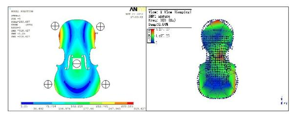
Fig. 4.8 Comparison of Mode 5 of the spruce plate by the FEM and the Modal Analysis
