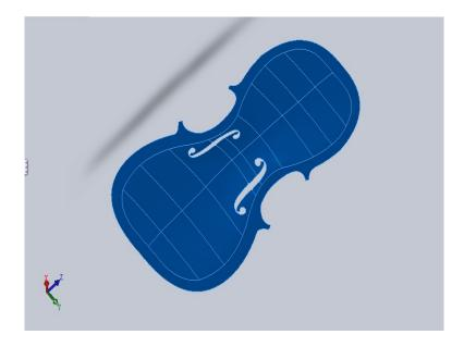
Fig. 3.3 CAD drawing of the spruce top plate
