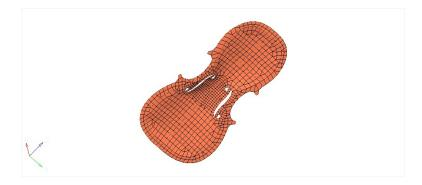
Fig. 3.4 Meshing of the spruce top plate
