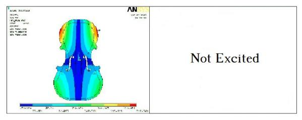
**Fig. 4.25** Comparison of Mode 1 of the composite plate #2 by the FEM and the Modal Analysis
