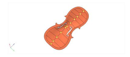
Fig. 3.2 A set of selected points for defining the arch height
