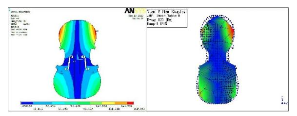
Fig. 4.18 Comparison of Mode 1 of the composite plate #1 by the FEM and the Modal Analysis
