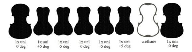
Fig. 4.10 Components of the second composite plate
