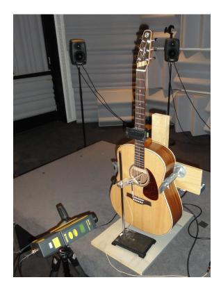
Figure 1: Experimental setup for input admittance and radiativity measurements.
