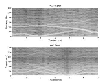
Figure 5: MIDI pressure signals from WX11 and WX5 wind controllers during upward hum.
