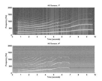
Figure 3: Pressure spectrograms as measured with All Sensors 1" and 4" devices during upward hum.
