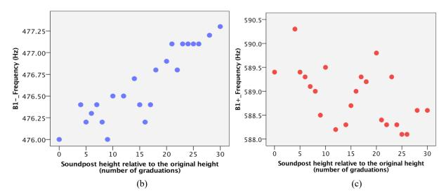
**Figure 5.10** Frequency for the A0, B1- and B1+ modes measured at different soundpost heights, ranging from 0 to 30 graduations (0.66 mm) relative to the original height of about 53 mm.
