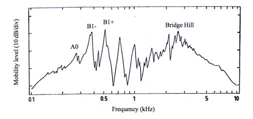
Figure 2.2 Bridge admittance of a Guarneri violin by Alonso Moral and Jansson [1982].
