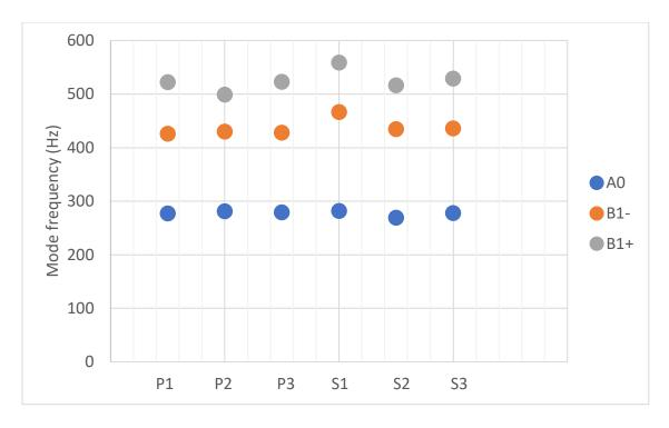
Figure 3.17 Frequencies of the A0, B1- and B1+ mode for the six violins.
