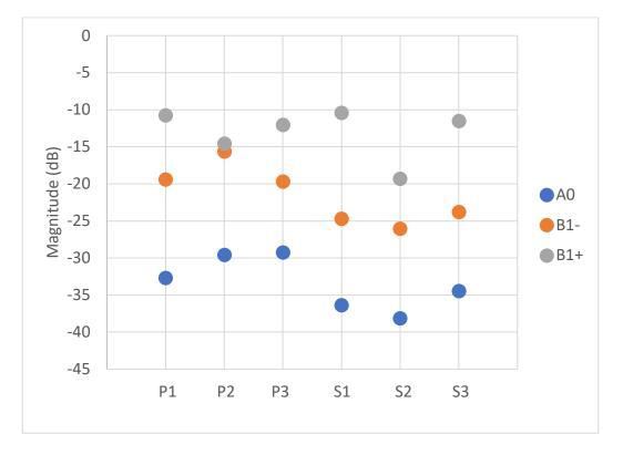
Figure 3.16 Magnitudes of the A0, B1- and B1+ mode for the six violins.
