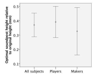
Figure 5.4 Mean optimal soundpost height relative to original height for all subjects, players and makers (errorbar = 95% confidence interval of the mean).
