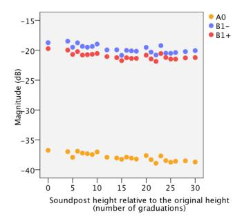
**Figure 5.9** Magnitude for the A0, B1- and B1+ modes measured at different soundpost heights, ranging from 0 to 30 graduations (0.66 mm) relative to the original height of about 53 mm.
