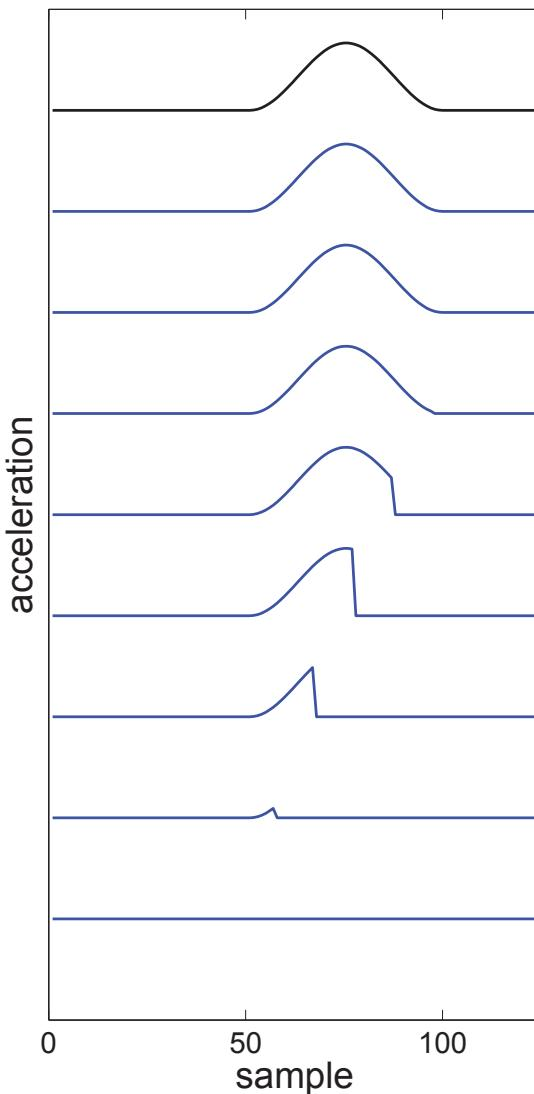
**Fig. 4.23** Updates of the RLS filter  $w(n)$ , temporally updated from the bottom to the top. The black one at the very top is the original signal.
