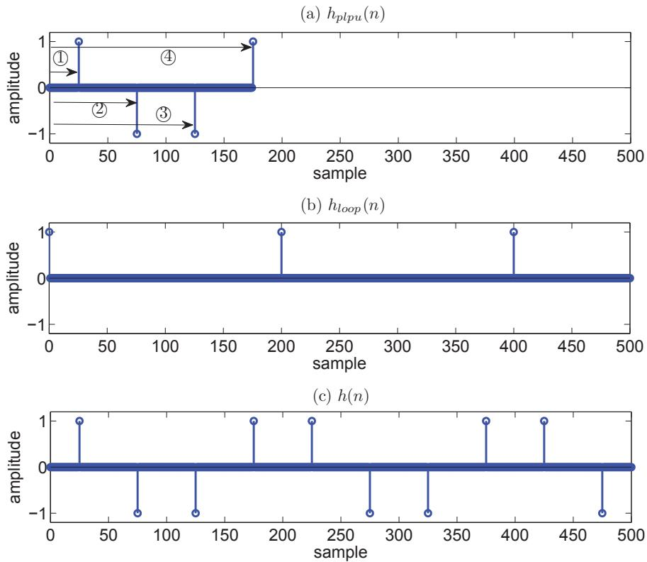
**Fig. 4.15** Impulse responses of  $H_{plpu}(z)$ ,  $H_{loop}(z)$  and  $H(z)$
