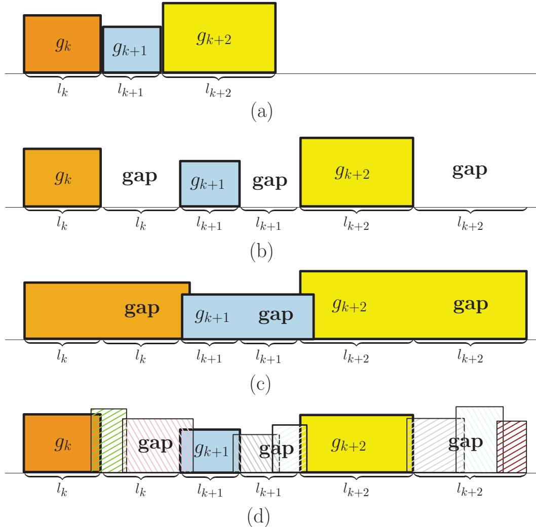
**Fig. 3.6** Time stretching and gap filling. (a) original sequence of grains  $g_k, g_{k+1}, g_{k+2}$  of length  $l_k, l_{k+1}, l_{k+2}$ , respectively. (b) time stretched with the time stretch factor  $\alpha = 2$ . (c) Gap filling with grain extension (d) Gap filling with additional grains.
