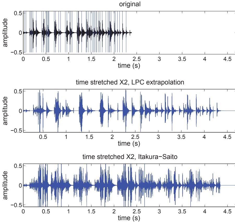
**Fig. 3.11** Time stretched clap sounds. a) Original sound. Blue vertical bars denote the grain boundaries. (b) Time stretched sound by a factor  $\alpha = 2$ , with the grain extension method. (c) Time stretched sound by a factor  $\alpha = 2$ , with the additional grain-based method (Itakura-Saito).
