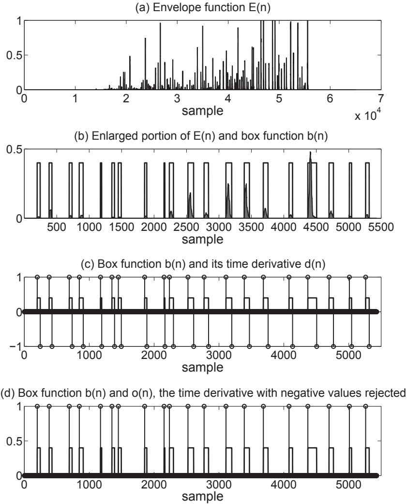
**Fig. 2.2** (a) Envelope function  $E(n)$  of given rolling sound  $y(n)$ .
