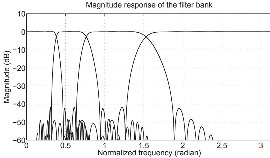
**Fig. 2.5** Magnitude response of the filter bank.
