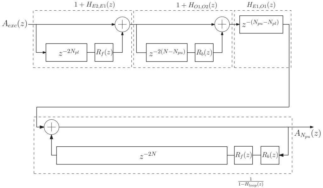
**Fig. 4.13** SDL model of the plucked string.
