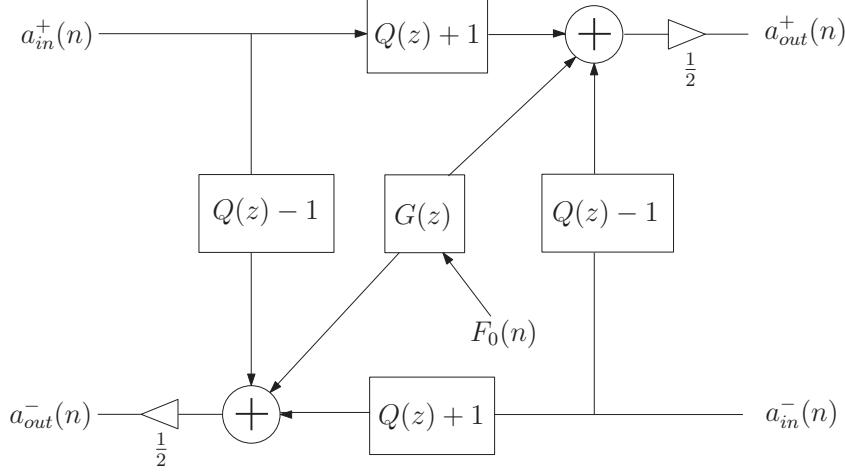
**Fig. 4.31** Scattering junction at the excitation point.
