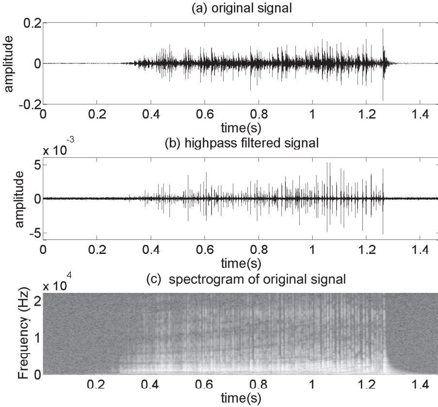
**Fig. 2.1** Top: Original rolling sound  $y(n)$ . Middle: High-pass filtered rolling sound  $y_{hp}(n)$ . Bottom: Spectrogram of  $y(n)$ .
