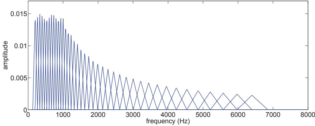
**Fig. 3.8** Triangular mel-scale filter bank from Auditory toolbox [1].
