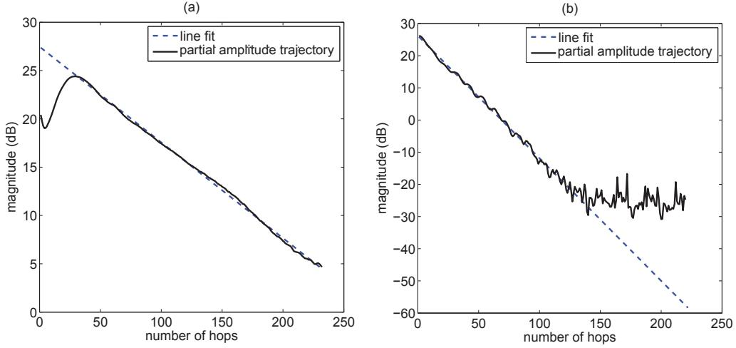
**Fig. 4.16** Line fit (dashed lines) of amplitude trajectories of partials (solid lines).  $f_0 = 147.85$  Hz and  $f_s=44100$  Hz. The hop size is 1024 samples. (a) 2th partial (295.41 Hz). (b) 11th partial (1635 Hz).
