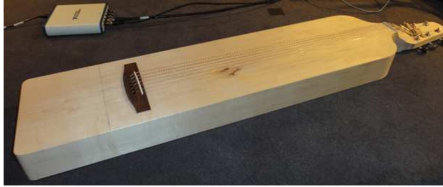
Fig. 2.9 The rigid base used to measure the Q factor of the guitar strings.
