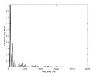
Figure 4: Normalized LTAS for the reed source signal simulated using physics model.
