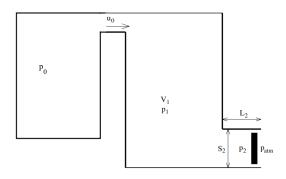
Figure 8: Adapted model with extra pressure chamber for bellows control
