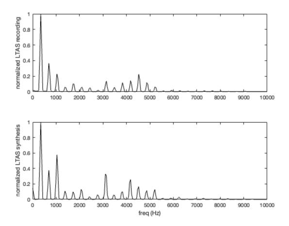
Figure 9: Comparison of normalized LTAS of a HQ-recorded note (top) and a synthesized note (bottom)
