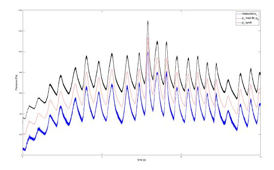
Figure 5: Reed chamber pressure measured using a pressure transducer (blue); median filtered version of raw reed pressure, also used as  $p_0$  for bellow simulation (red);  $p_1$  simulated using the proposed model(black);  $p_0$  and simulated  $p_1$  plots shifted in y axis by 150 Pa and 300 Pa for better visibility
