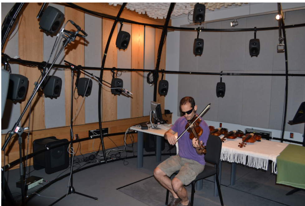
Figure 5.2 Recording setup: two cardioid microphones configured in X-Y stereo coincident position and one free-field microphone.
