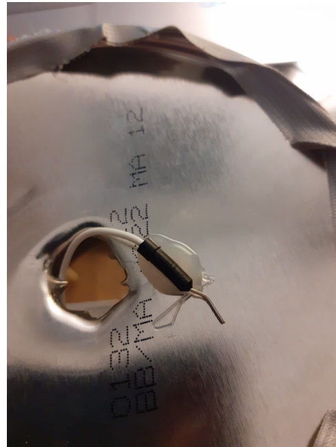
Figure 3: A close up the hole punched through the base, and the hot glue used to connect a wire from the metal plate to the rest of the circuit
