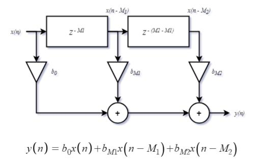
This system was ultimately utilised in the internal components of the resonant body model, where tapped delay lines are used shortly before a feedback element to further the sense of internal reflection.
