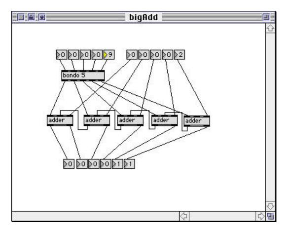
Again the digits are restricted. You can make the numbers as big as you want by adding adders. (You used to be able to get little mechanical calculators that worked this way.)
