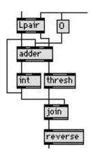
The adder is the same one used above. It will work sequentially if we just feed the carry back in. Of course we have to clear the carry before the addition starts, hence the 0 in a box. The carry also becomes the first digit of the number, even if it is zero. Thresh collects the sum into another list, which is still backwards. Join tacks the carry on and the list is reversed.
