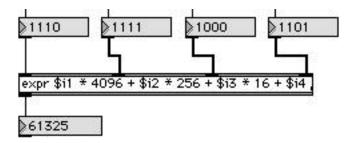
Notice the magic numbers for 4 bit nibbles are 4096, 256, and 16. These are the divisors you would use if you prefer the division method of nibblizing. (The binary operators are a bit faster, but unless you are doing thousands of conversions, the speed difference is not noticeable.)
