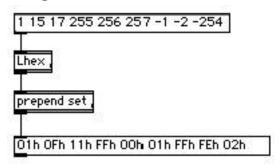
Llong turns the hex symbols back into numbers. If the original number was masked by Lhex, long can't know it and returns the modified value. Note that one digit symbols must be written 01h. Llong can deal with hex numbers of any sizeup to FFFFFFFh (which is –1 in a 32bit int).
