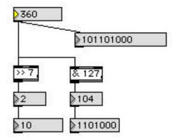
These use binary operators. >> 7 is right shift 7 steps, which directly carves off 7 bits. The bitwise AND (&) is also known as masking. When a bitwise AND is performed on two numbers, the result will have 1s only where both of the operands have 1s. As an example,
