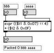
I mask the input values to keep them within range. If a user entered a 5 bit value for aaaa, it would also change bbb, which might be very hard to track down. The parentheses are required to make sure the steps are performed in the correct order.
