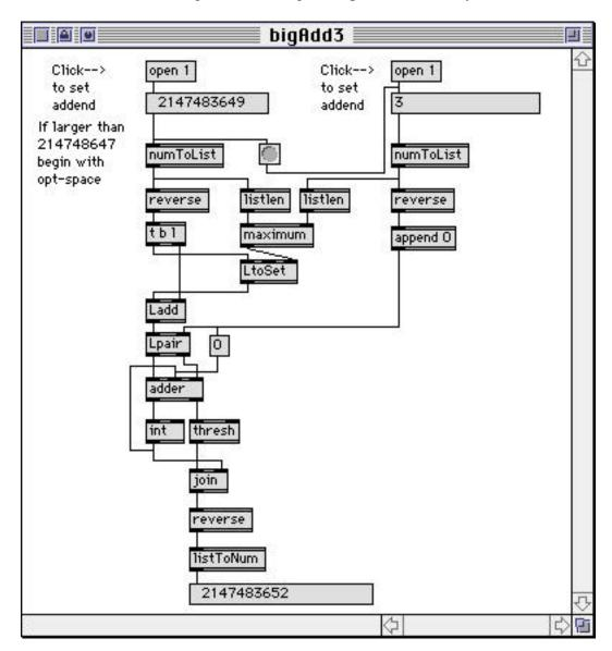
The numToList subpatcher converts whatever is entered into the message box into a list of digits. The message box will try to make a number out of any entry that is all digits and spaces, so for large numbers you must include some other character. The non breaking space will display nicely. NumToList strips these out:
