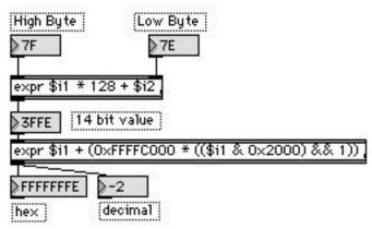
What we are doing is looking at the most significant bit of the incoming number with the mask 0x2000. If it's a one, the number is negative and we add the magic value 0xFFFFC000. That immense number will fill the leading bits of the incoming number with 1s to create a 32 bit negative.
