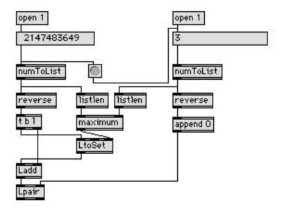
The adder will need to receive the lists least significant digit first, so the lists are reversed.
