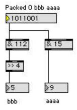
The masking value for the upper bits (4-6) is found by adding the power of two each bit represents. In this case, 16+32+64=112. Building such numbers is easily done with expr:
