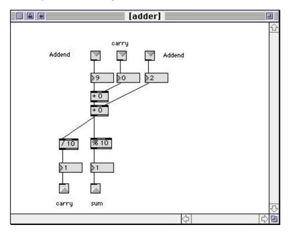
The number boxes for the addends are restricted to 0-9, the carry input is restricted to 0 or 1. This accepts two addends and a carry, and produces a one digit sum and a carry of 1 or 0. You'd put it in an addition patch like this:
