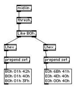
A problem when dealing with sysex is detecting particular messages when they come into the computer. Usually, a message is identified by a "header", the first few bytes of the data. Like is a object that tests the incoming list against its arguments, and passes the list out the left if they match. If no match, the list goes out the right. Here it's looking for control messages on channel 0, passing pitch bends on for another Like to deal with.
