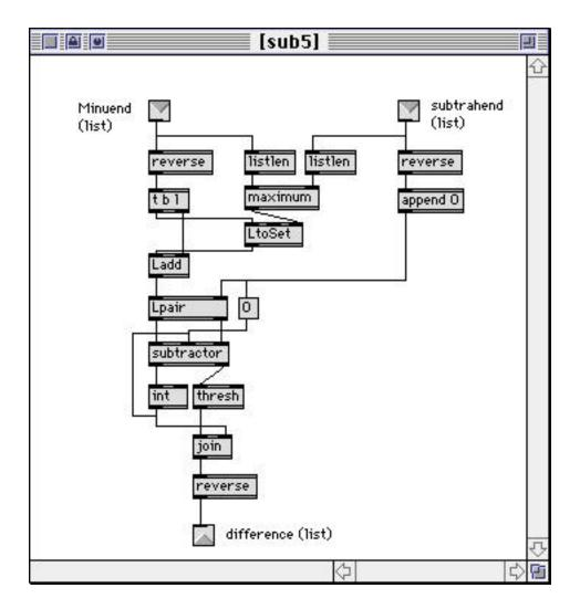
Actually, it's another subpatch. You'll see why in a moment. It is taken directly from the middle of the addition patch above, with a subtractor replacing the adder. It expects input in the form of digit lists as before.
