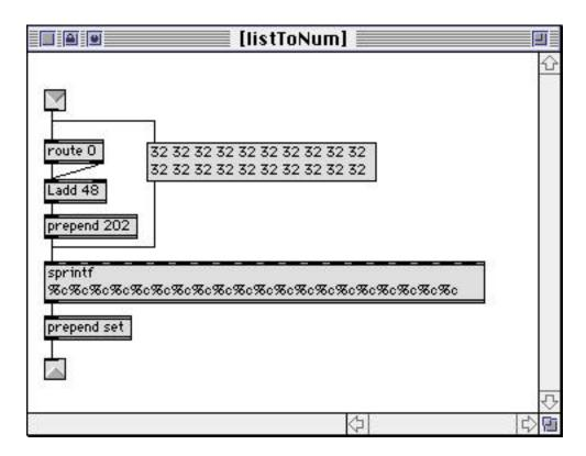
Route 0 is used to strip off the leading 0, if any. The prepend 202 starts the list with a non-breaking space. The list of 32's clears sprintf, in case the number coming in is shorter than the last one.
