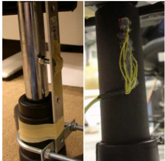
Figure 6: Mechanical shaft encoder (left) and optical shaft encoder (right)
