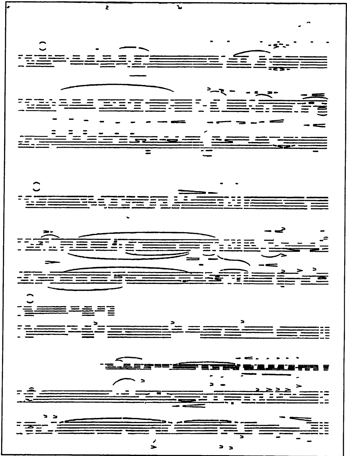
Figure 4.12 Connected-components narrower than staffspace_height removed.
