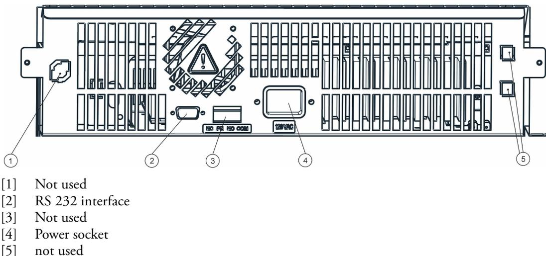
**Figure 4-7 Signal Interfaces and Power Socket**
