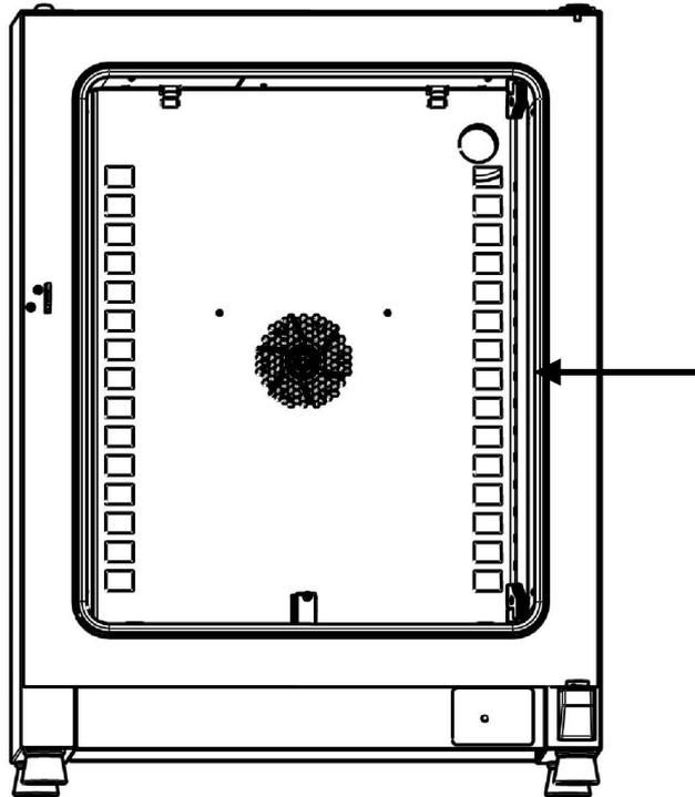
**Figure 10-1 Door Seal Replacement**
