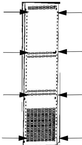
**Figure 5-8 Removing the left and right support profiles**
