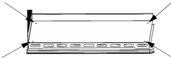
**Figure 5-7 Removing the bottom plate**
