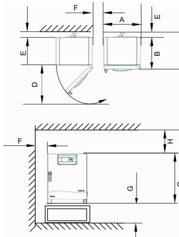
**Figure 3-1 Table-top incubators, dimensions and required clearances**
