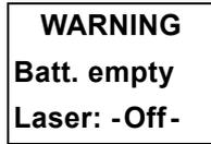
*The laser has been switched off because the battery is empty. To avoid completely draining the battery and thus shortening its useful life, set the rocker switch of the battery charger in the direction of the charge level indicator. Then reload the battery as described in [section A.1.2](#) under Charging battery.*
