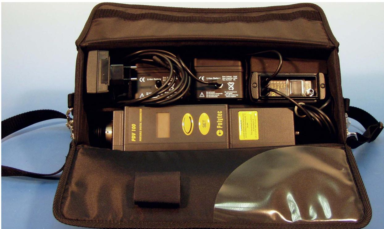
Figure A.1: Carrier bag PDV-BS with battery, battery charger and PDV 100
