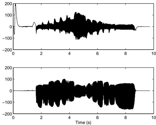
Figure 2. Waveform of the upstream pressure (top) and downstream pressure (bottom) during an ascending and descending overtone series from F3 (175 Hz) to F5 (700 Hz).
