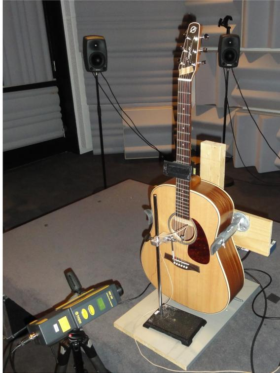
Figure 1: Experimental setup for input admittance and radiativity measurements.
