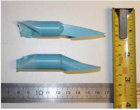
Figure 12. Silicone molds were used to get the internal geometry of the mouthpieces. From top to bottom : the mold corresponding to the Selmer mouthpiece, and that corresponding to the Lebayle mouthpiece.
