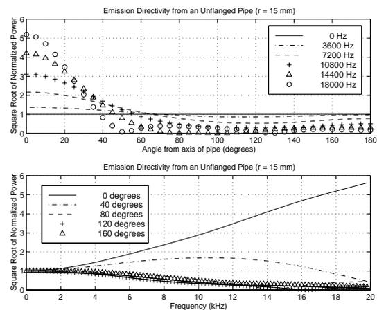
Figure 3: Sound emission directivity at the open end of a cylindrical pipe.
