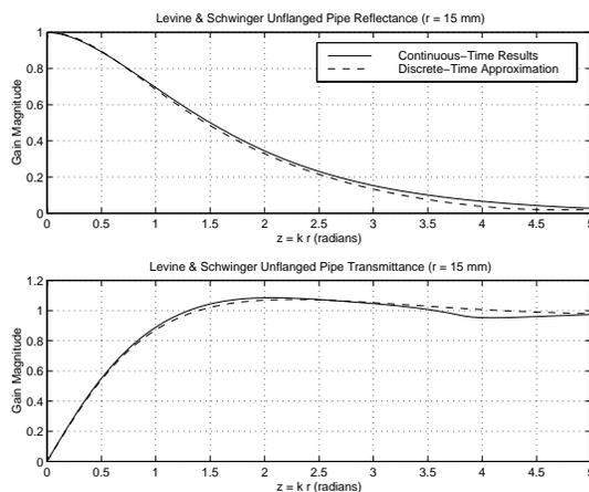
Figure 2: Sound reflection/transmission at the open end of a cylindrical pipe.
