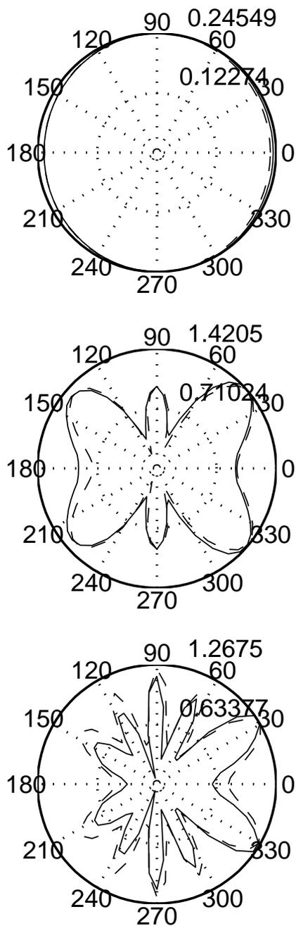
Figure 5: A comparison of the DW results (-) to the frequency-domain calculations (- -) of Rousseau (1996) for a six hole air column (three finger holes open, three finger holes closed). (top) 506 Hz; (middle) 2842 Hz; (bottom) 4845 Hz.
