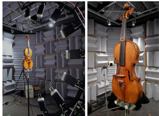
FIG. 1. (Color online) (Left) Semi-circular 60-microphone array used for violin radiation measurements. The violin is held on the pole attached to the rotating base. (Right) Detail of the rig used for holding the violin, along with the arm to which the impact hammer pendulum is attached.
