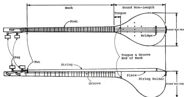
Figure 1: The schematic view of the setar [4].
