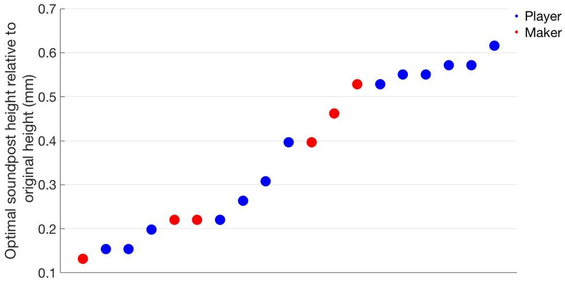
**Figure 5.2** Optimal soundpost height relative to original height for every subject sorted from smallest to largest.
