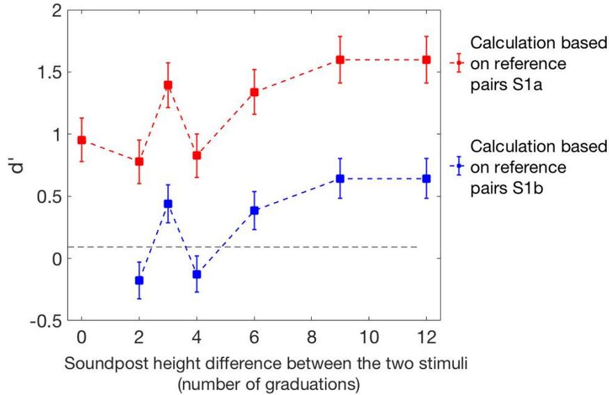
**Figure 6.6** Perceptual sensitivity  $d'$  for each  $|\Delta H|$  calculated using two sets of reference.
