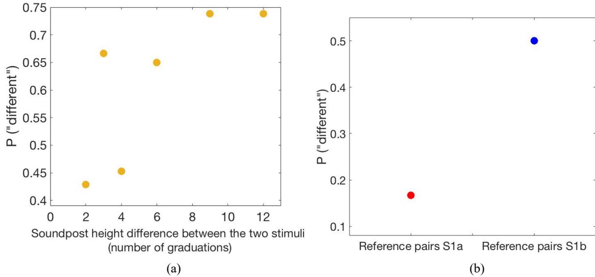
**Figure 6.5** Probabilities that subjects considered each pair of stimuli as different, when the pairs consisted of recordings made at two different heights (a) or at the same height (b).
