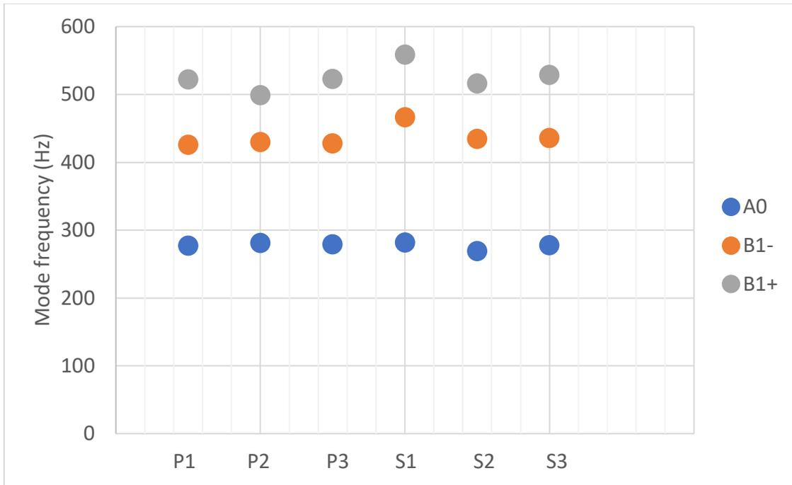
**Figure 3.17** Frequencies of the A0, B1- and B1+ mode for the six violins.
