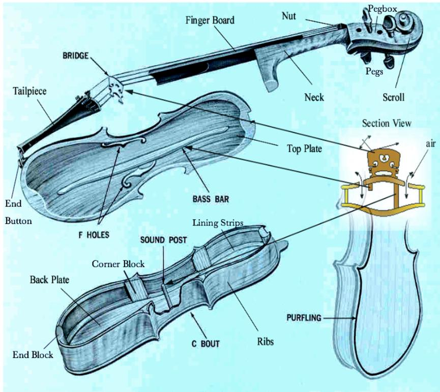
**Figure 2.1** Exploded view of violin showing the components by Hutchins [Hutchins, 1967; Zhang, 2015].
