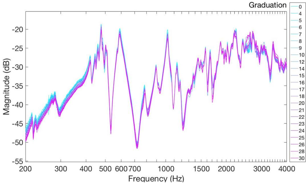
**Figure 5.7** Bridge admittance measurements on the violin used in the soundpost height playing test for different soundpost heights. Soundpost height was represented relative to the original soundpost height (about 53 mm) by number of graduations. The colour scheme is shown in the legend: from the original soundpost height (0 graduation) to the highest soundpost height (30 graduations), the soundpost height was denoted by gradient colour from blue to magenta.
