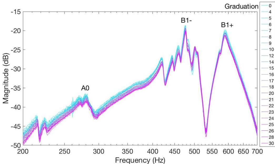
**Figure 5.8** Enlarged Figure 5.7 particularly between 200 and 700 Hz with three signature modes identified and labeled. Soundpost height was represented relative to the original soundpost height (about 53 mm) by number of graduations. The colour scheme is shown in the legend: from the original soundpost height (0 graduation) to the highest soundpost height (30 graduations), the soundpost height was denoted by gradient colour from blue to magenta.
