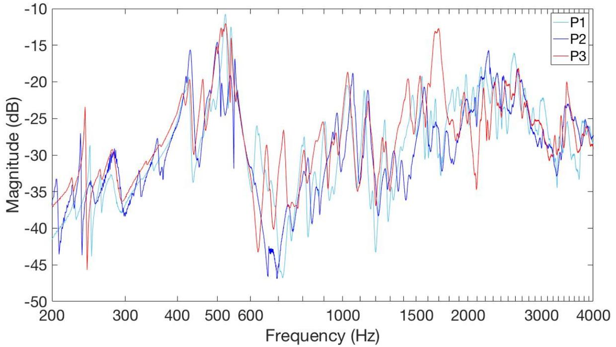
**Figure 3.13** Measured bridge admittances of performance violins.
