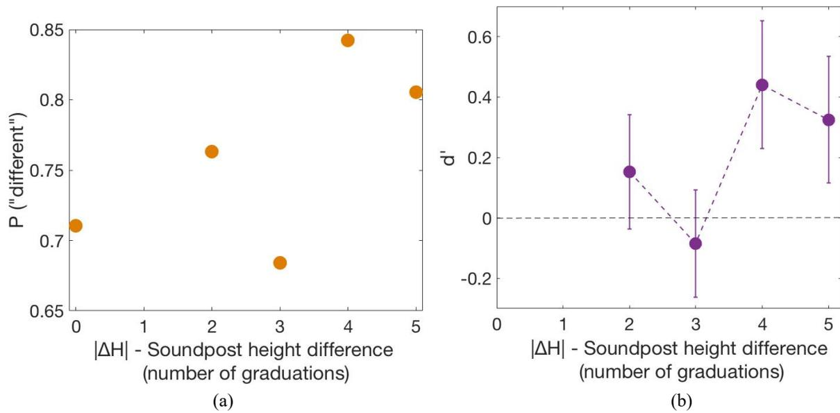
**Figure 5.5** (a) Probabilities subjects considered the two soundpost heights with a height difference of  $|\Delta H|$  as “different”; (b) perceptual sensitivity  $d'$  for each  $|\Delta H|$  (error-bar = 95% confidence interval around  $d'$ ).
