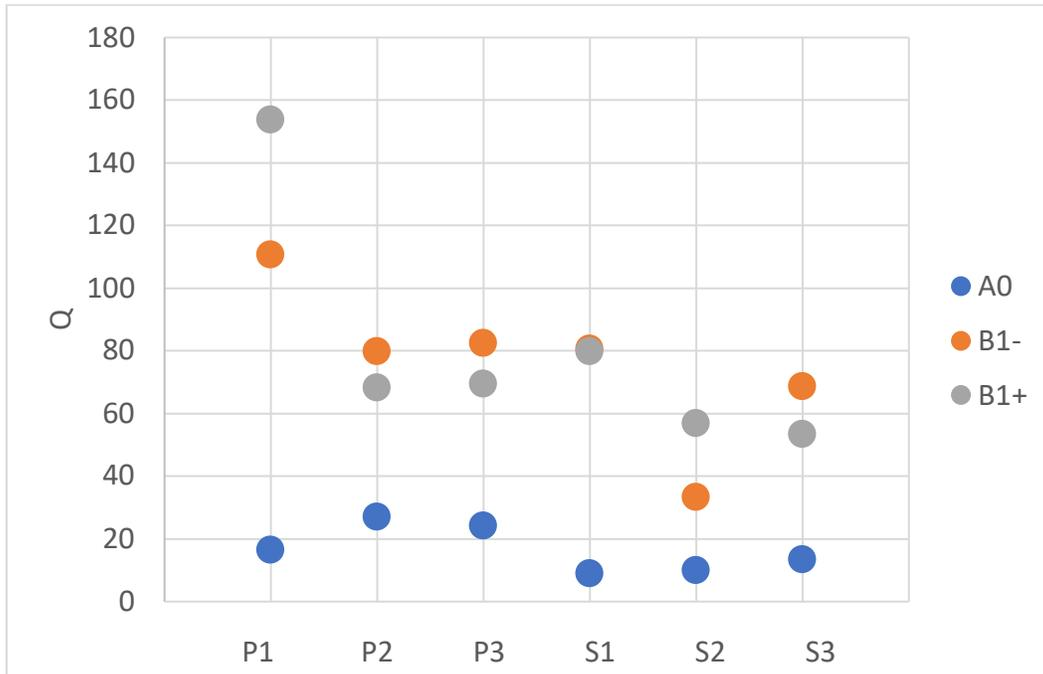
**Figure 3.18** Q values of the A0, B1- and B1+ mode for the six violins.
